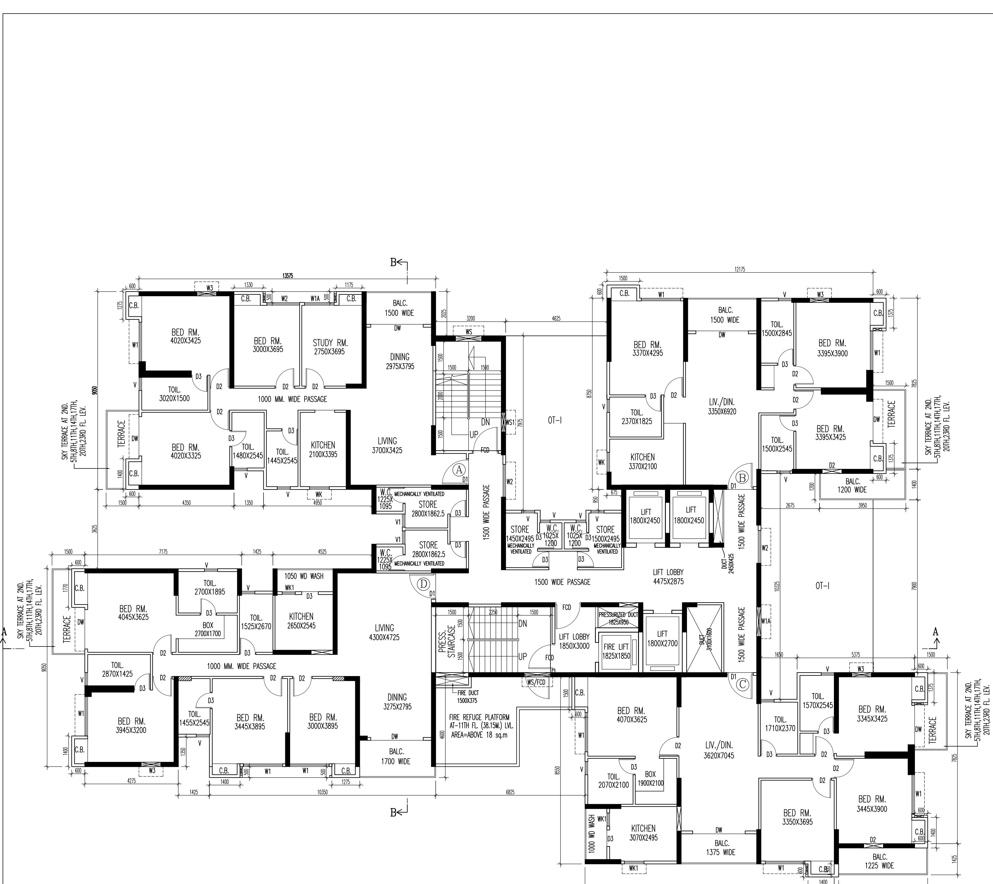
TYPICAL (2ND,5TH,8TH,11TH,14TH,17TH, 20TH,23RD) FLOOR PLAN BLOCK - A
